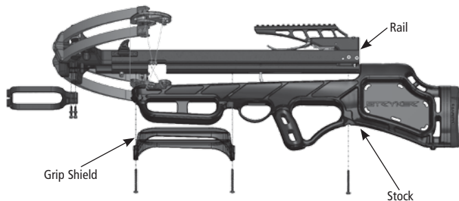
Figure 2: Positioning and attaching the rail, grip shield, and stock.
