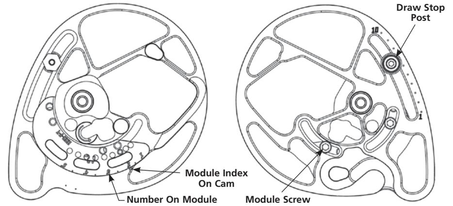
Figure 2: Conventional Binary Draw Length Adjustment
