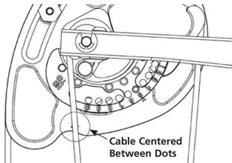
Figure 3: Cam Timing
