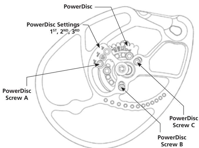
Figure 2: PowerDisc Adjustment
