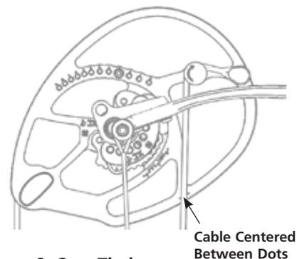
Figure 6: Cam Timing
