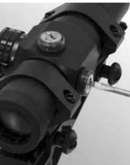
The standard targeting scope uses three reticle red dots to represent distances of 20, 40, and 60 yards. Two calibrated screws on the scope allow you to adjust sighting. The top screw adjusts horizontally (windage); the side screw adjusts vertically (elevation).
